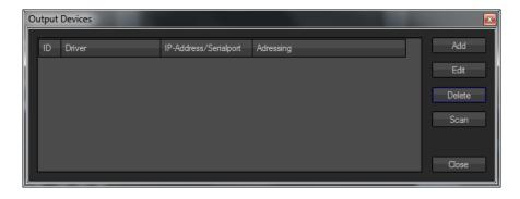
On the left side you can see already configured devices with its main parameters, on the right side you get the control buttons to add, edit or delete a new device. Additionally you can use the Scan button to search within your network for Art-Net nodes. Any found and useable Art-Net node will automatically be configured and added to the list.
