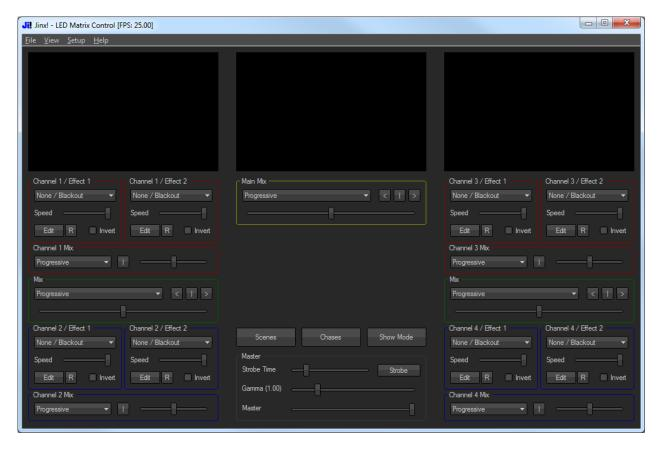
Every effect channel is divided into 2 identical effect generators with a crossfade/mix section at the bottom where you can mix the animations that are generated by the independent generators.
