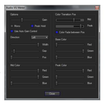
With the direction option you can choose the direction your bars will follow on your matrix. To use the VU Meter as additional effect to use as overlay, you can define the width of the bars as well as the gap between (in stereo mode) and the position on the matrix. So it is possible to create small bars which will stay at the edges of your matrix (with a huge gap) or you can use really huge bars as full screen. You can even use a single bar to animate a led stripe.
