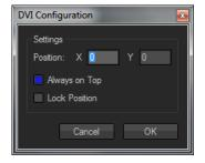
The DVI Configuration window can also be started over the menu with **Setup -> Configure DVI Window**. Here you can set the Always on Top and the Lock Position features as well. Additionally you can set the position of your DVI Window exactly by given the corresponding pixels. The pixel count will start with 0 on the upper left corner.
