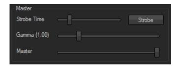
The most important fader is the Master fader at the bottom of this section. This will control the main brightness. So if your matrix is too bright into a small room you can use this fader to dim it down to an eye-friendly level. If you double click on the label, the fader will jump to 0% brightness.
