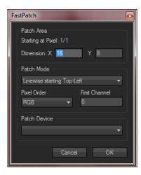
The fast patch will assign ascending channel numbers within a device to the next pixel, corresponding to your matrix controller and setup you can patch the whole matrix at once or single areas.
