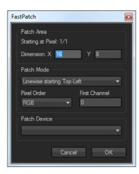
The Fast Patch starts with the actually marked pixel. Now you have to set the dimension of the block you want to patch, choose the correct output device, the pixel order and the first device channel. To do the patch you simply have to click the OK button.
