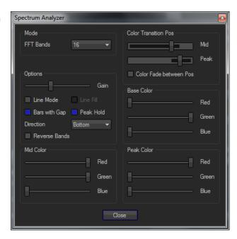
There are multiple options available for the spectrum analyzer. You can get a clear picture by activating gaps between the bars and even can enable or disable a peak hold feature.
