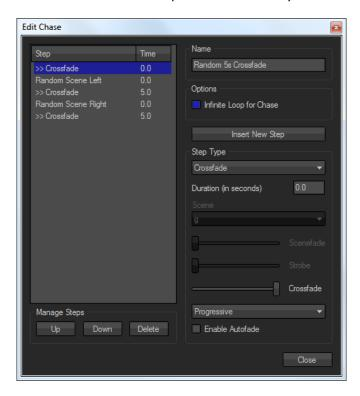
The chase editor is clearly structured. On the left side you see the step list with the well-known Up, Down and Delete buttons below it. On the right top you can change the name of the chase and set the chase to an infinite loop, which means the chase will never stop and automatically start the first step after reaching the last.
