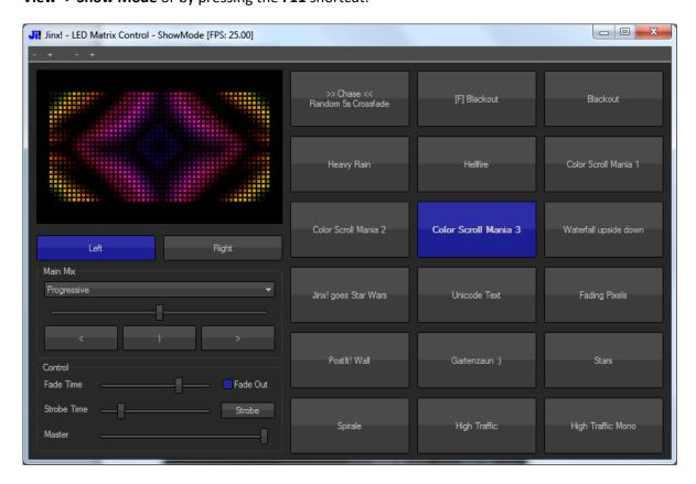
With the show mode window you have a touch screen friendly screen to control all the stored scenes and chases which will be shown as buttons. The show mode window is fully resizable and the buttons get automatically placed and ordered, starting with all chases and followed by the scenes. The size of the buttons can also be adjusted with the small – and + buttons inside the top menu. The first pair will control the width and the second pair the height of all buttons.
