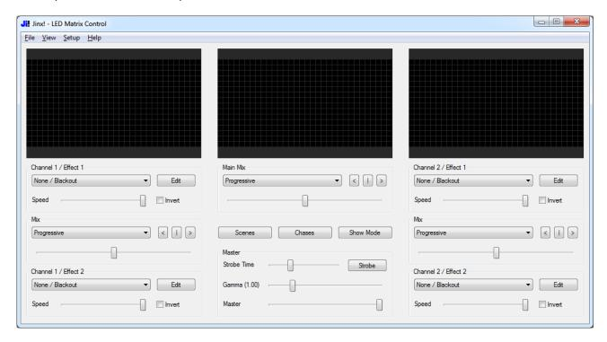
Every effect channel is divided into 2 identical effect generators and a crossfade/mix section in between where you can mix the animations that are generated by the independent generators.
