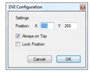
The DVI Configuration window can also be started over the menu with **Setup -> Configure DVI Window**. Here you can set the Always on Top and the Lock Position features as well. Additionally you can set the position of your DVI Window exactly by given the corresponding pixels. The pixel count will start with 0 on the upper left corner.
