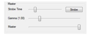
The most important fader is the Master fader at the bottom of this section. This will control the main brightness. So if your matrix is too bright into a small room you can use this fader to dim it down to an eye-friendly level. If you double click on the label, the fader will jump to 0% brightness.
