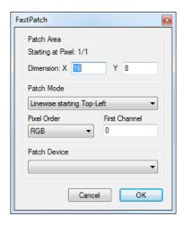
The Fast Patch starts with the actually marked pixel. Now you have to set the dimension of the block you want to patch, choose the correct output device, the pixel order and the first device channel. To do the patch you simply have to click the OK button.
