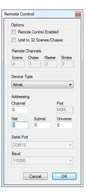
The second area will display the 4 controls and tell you the actual channel they are using. The channels will always be ascending and the control order is fixed. The start channel can be set inside the protocol addressing area.
