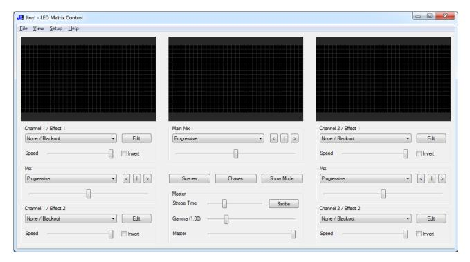
Every effect channel is divided into 2 identical effect generators and a crossfade/mix section in between where you can mix the animations that are generated by the independent generators.
