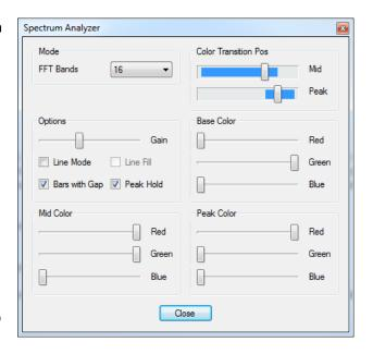
There are multiple options available for the spectrum analyzer. You can get a clear picture by activating gaps between the bars and even can enable or disable a peak hold feature.
