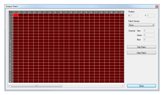
Inside this window you can see and scroll through every single pixel of your defined matrix. Every pixel will show you its actual state. If it's marked red its unpatched, means no output device and channel is assigned, if it's already patched it will be marked green.
