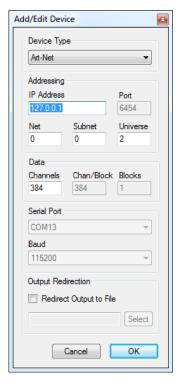
This dialog has various options which are not all useable by every device type. In the first section you can choose the device type you want to configure, the next section will help you to address the device if it's a network based protocol.
