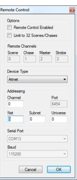
The second area will display the 4 controls and tell you the actual channel they are using. The channels will always be ascending and the control order is fixed. The start channel can be set inside the protocol addressing area.
