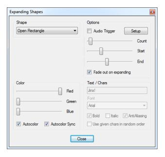
As already said, this effect can be controlled by audio. This means with every audio trigger a new shape will be started and begins to expand and fade. After activating the audio trigger you have to setup your trigger frequency, threshold and gain. You will find more about this in the "Audio based Effects" chapter inside this manual.
